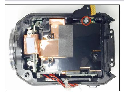
Once the circuit board is removed, you will want to remove the Phillips screw (3mm headsize x 2 mm length) near the ribbon cable. ONLY REMOVE THIS ONE SCREW.
