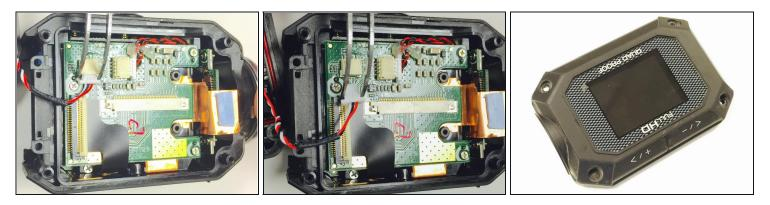
• Now take out the connector by pulling the white clip out of the casing (as shown in the photos). This will will disconnect the screen from the main cable, allowing you to attach your new LCD cover.
