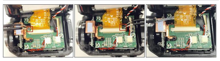
• Using the tweezers, carefully push up the left and right sides of the cable ribbon clip. Use the tweezers to life up and remove the clip.
