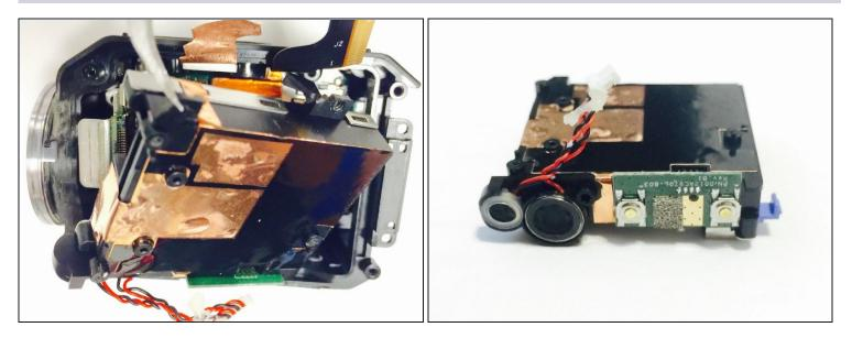
• Now you should be able to gently remove the battery housing out of the device. If you are having difficulty getting the battery housing to come out, you may want to use the plastic opening tool to help get it started.
