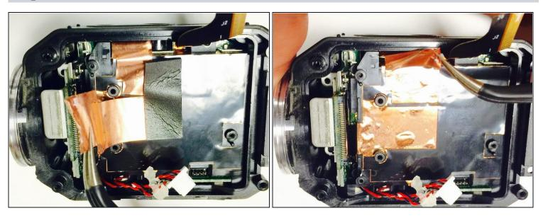
• Carefully remove both the top and bottom copper strips by gently pulling them off with the tweezers.
