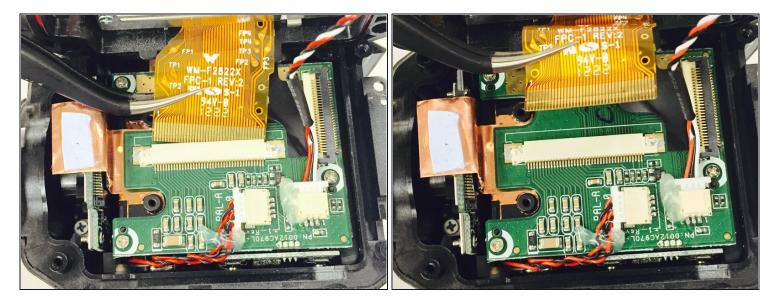
• Using the tweezers, carefully remove the ribbon cable by gently grasping it and pulling up.
