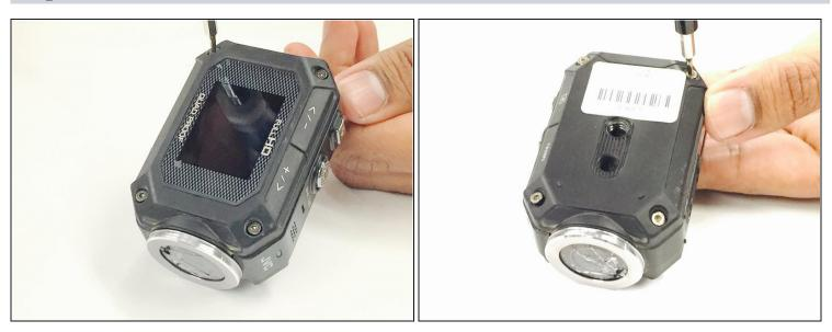
• Using a 1x1xH1.5 torx screwdriver, remove the 8 screws (5mm headsize / 4mm length) from the corners of both the front and back of the camera (4 screws on each side).
