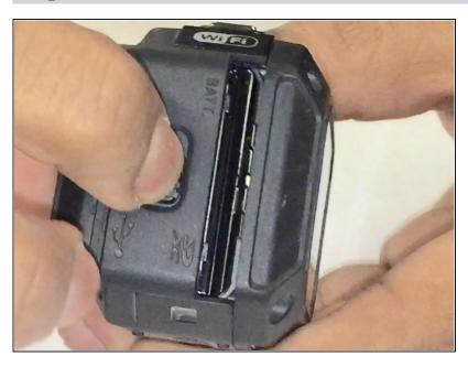
• While still pushing down on the black switch, slide back the battery cover (see photo for direction).
