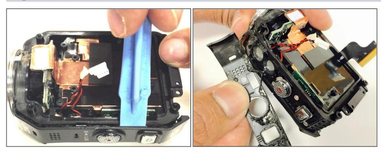
• Use the plastic opening tool to gently remove the top cover from the camera. It is glued on, so you may need to work at it to get it to come off.
