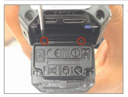
After removing the battery, take out the two Phillips screws (4mm headsize x 3mm length) screws. You can now remove the battery cover.
