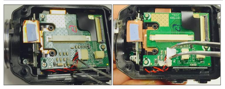
• Carefully peel off the glue holding the red and black braided wire down to the circuit board. Then remove the connector by gently pulling it out of its casing. You will want to save this glue as it may come in handy when re-assembling your device.
