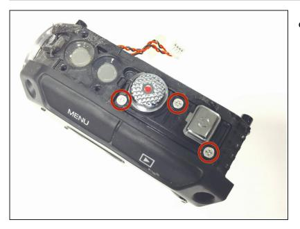
• Once the cover has been removed, you will want to remove the three Phillips screws (2mm headsize x 2mm length) that are underneath.
