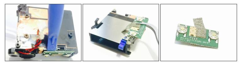
• The power and record buttons are glued to the battery housing, so use the plastic opening tool to gently pry off and remove the buttons.
