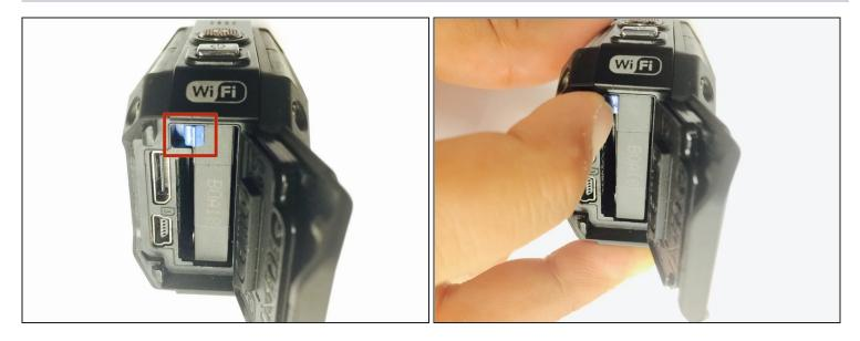
• Push the cover up to open the battery compartment, and then push the blue battery release switch.
