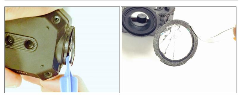
Use the plastic opening tool to gently pry the lens off of the camera.
