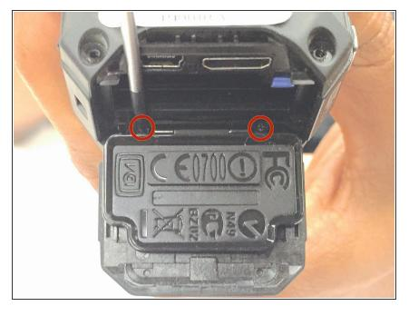
After removing the battery, take out the two Phillips screws (4mm headsize x 3mm length) screws.
