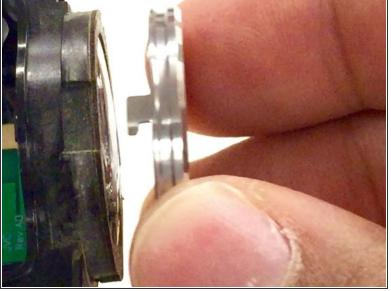
Twist the metal ring on the lens to the right and then pull it off.
