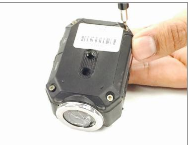
• Using a 1x1xH1.5 torx screwdriver, remove the eight screws (5mm headsize / 4mm length) from the corners of both sides of the camera (4 screws on each side).
