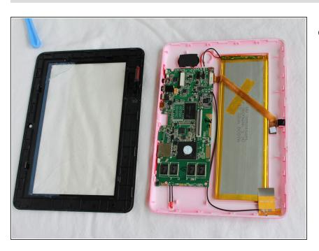
Remove the cable from the motherboard.
