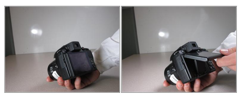
• Lift up the screen so you can access the back of the screen.
