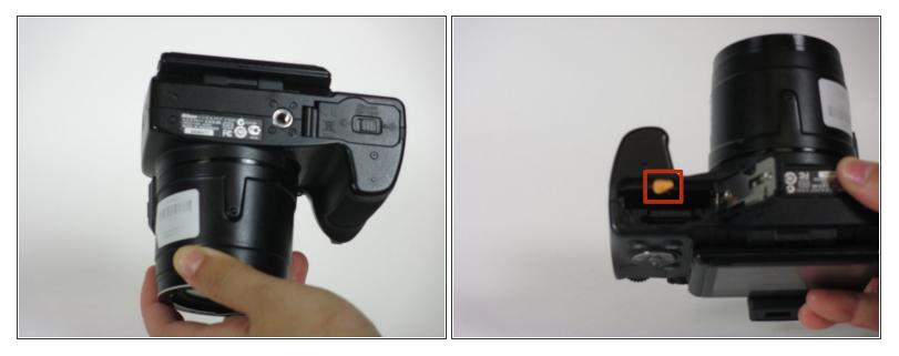
A Electric shock is a huge risk if the battery is not removed while taking the camera apart.
