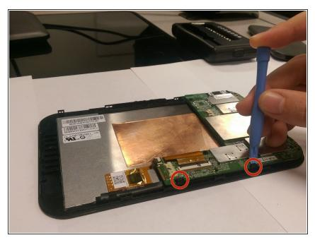
• Remove the circuit board by gently coaxing it from the clips located just to the right of the circuit board.
