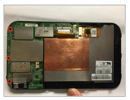
Remove the the remaining 3 screws to unfasten circuit board. Keep the screws.
