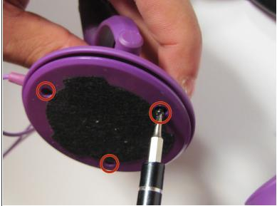
• Use the small Phillips screwdriver to remove three 8mm screws on the surface of the earphones.
