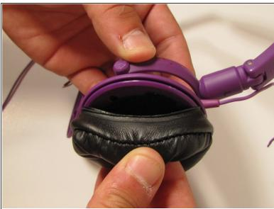
Pull the edge of the pad where it meets the plastic of the ear-cup to separate the padding from the ear pad.
