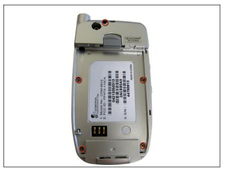
Remove the five (5) total screws using a Philips head screwdriver.
