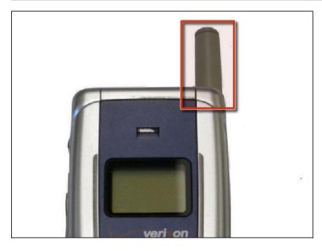
Locate the antenna (shown in red box) at the top of the phone when closed.
