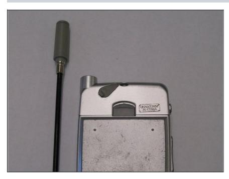
Using your thumb and index finger, grip the antenna near its base and unscrew counter clockwise. Once loose, remove the antenna by pulling it from its insert hole.
