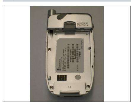
The back of the phone will look like this when the battery is correctly removed.
