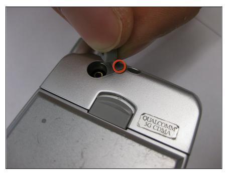
Remove the screw that sits underneath the rubber covering.
