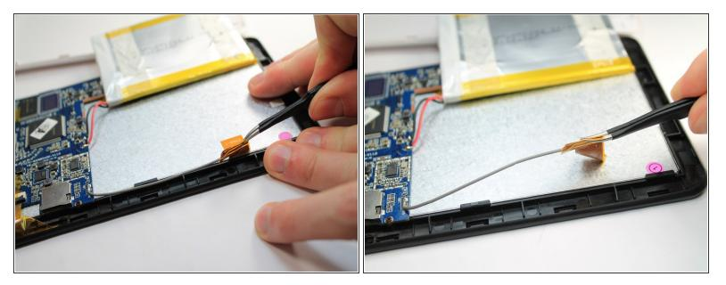
• Gently peel the WIFI Antenna up using a pair of tweezers.
