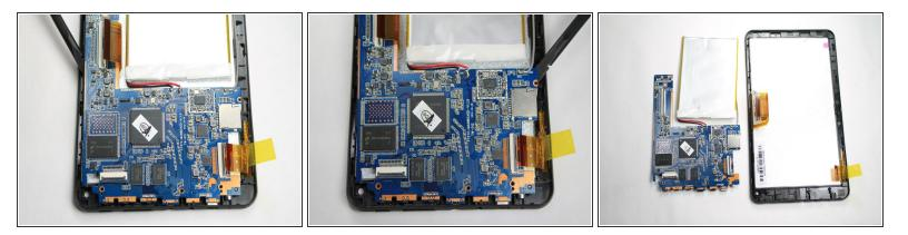
• Gently slide the spudger below the logic board at the left side nearest the battery. Lift upward and away from the power button and bottom connectors.
