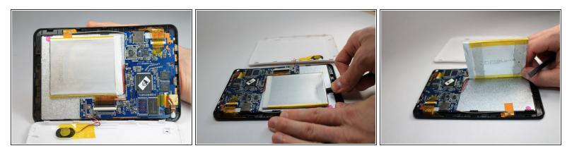
Use flat side of the spudger to get under battery and use pressure to release from glue. Do this all the way around battery until it comes off.
