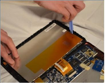
Insert the plastic opening tool into the wedge and pry it open.
