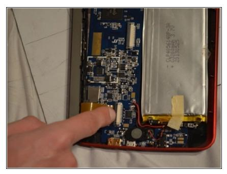
After you remove the digitizer, open the latch and remove the screen.
