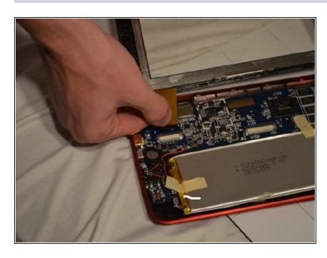
To install the new screen, insert the digitizer into the new screen and latch them back in.
