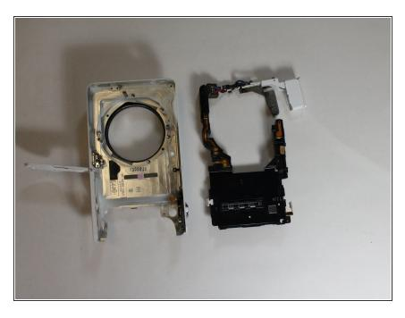
• Pull the flash and battery case out of the device.
