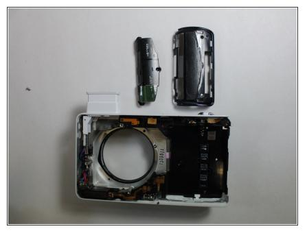
• The black plates on the other side can be removed after these screws.
