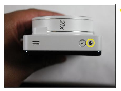
• Turn the device and remove the additional 3/16" screw.
