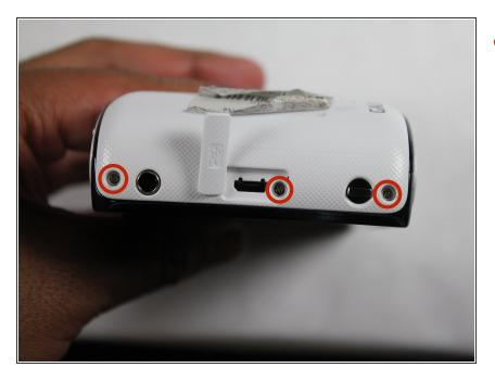
Begin removing the 3/16" screws for the device.
