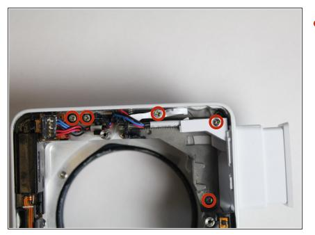
Remove all the screws circled. There is 1 1/8" screw by the flash, 1 9/32" screw that holds the flash button, 2 5/32" screw that is on the grey frame for the flash, and 2 5/32" screws that holds the cable frames on the top left.
