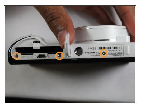
• Turn the device and remove the additional 3/16" screws.
