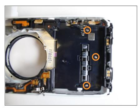
• Unscrew the 3 5/32" screws that cover the battery plate.
