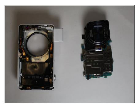
• Lift the motherboard and lens out of the case.
