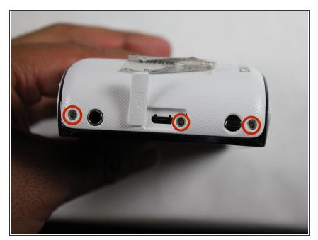
Begin removing the 3/16" screws for the device.
