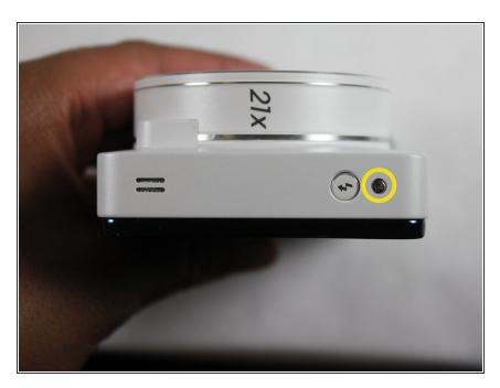
Turn the device and remove the additional 3/16" screw.
