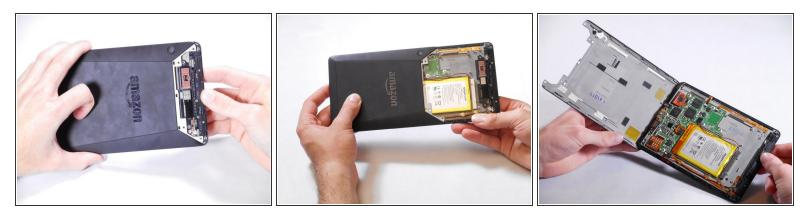
• Once the screws are removed, the back panel can slide off the device.
