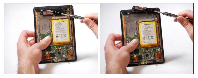
• Remove the magnetic component with the magnetic head of the aluminum driver.
