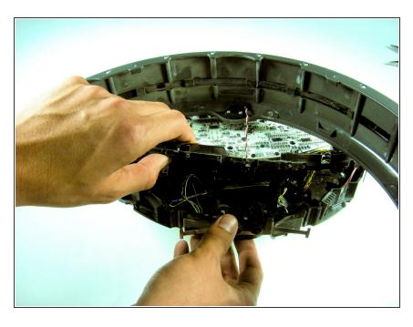
Remove the round cliff sensor belt by pulling it up off of the front edge of the Roomba.
