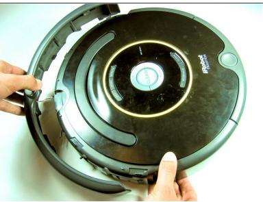
Remove the front bumper. You may remove it with your hands or a tool. It should snap off with some effort. It will still be attached to the Roomba by a couple of wires.
