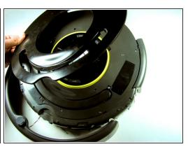
Remove the top plastic cover by first using a plastic opening tool or metal spudger around the edges. Then, carefully lift up from the back.
