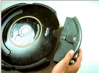
Pull out the bin while pressing down on the release button. Set aside.
