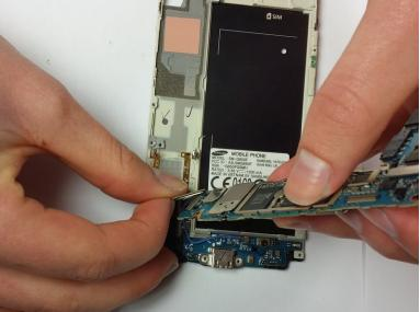
Find the end of the blue piece shown in the picture and gently lift the top of the part away from the casing.
