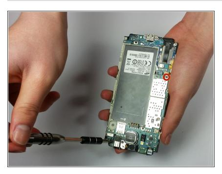
Using the Phillips #00 screwdriver remove the two 3mm screws.
