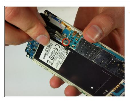
Finally, remove the last connector that is attached by a blue cable.
