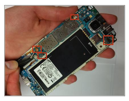
Using your fingers or a Metal Tweezer, apply slight pressure and pry up each of the four pin connectors shown in the picture.
