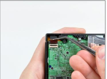
• Use your fingernail or the edge of a plastic opening tool to carefully flip up the dual camera ribbon cable retaining flap.
