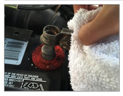
Using a rag, place the positive terminal back onto the positive node.
