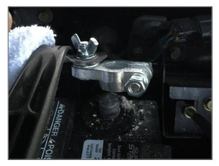
Place the negative terminal back onto the negative node.
