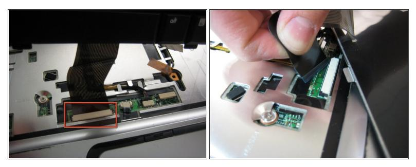
• Remove the ribbon from the computer by pulling straight back (away from the track pad and towards the monitor).
