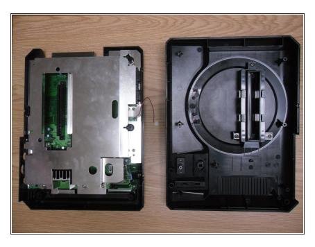
Separate the main board from the outer case.
