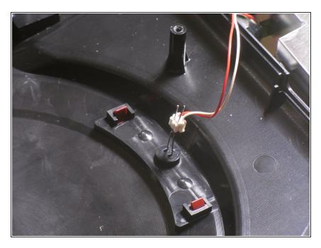
Bend out the LED leads into vertical positions.
