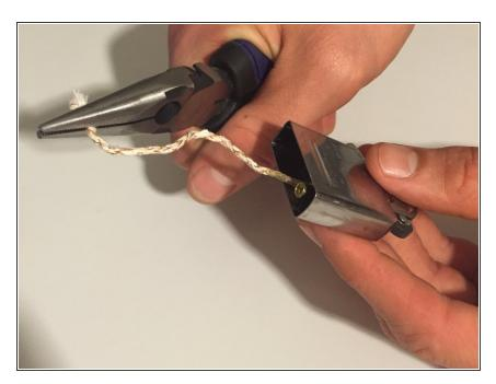
Remove the spent wick by pulling down with the needle nose pliers through the bottom of the lighter.
