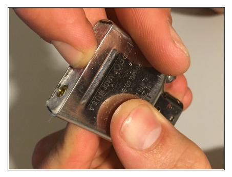
Replace the felt pad by gently pressing it back into place.
