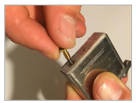
Replace the flint by putting it back down the flint tube and screwing the flint spring back into place.
