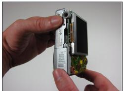
Firmly grasp the back of the camera and pull the away the casing.
