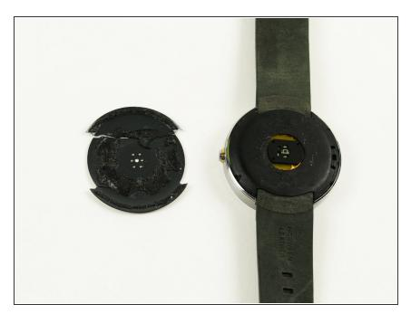
Once the adhesive has been successfully loosened, gently pull the rear cover off.
