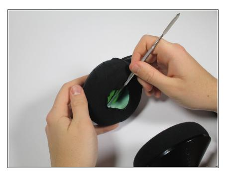
Carefully slide the spudger between the ear pad and the speaker cover, along the seam, to remove the adhesive.
