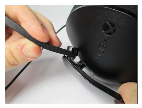
Lift the joint of the boom up and over its pivot point to separate the microphone from the headset.
