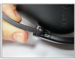
Use the flat end of a spudger to pry out the rubber stopper at the base of the boom.
