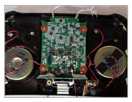
Using the Phillips #1 screwdriver, remove the four 10mm screws from the corners of the motherboard.
