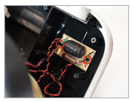
Using a Phillips #1 screwdriver, remove the two 7mm screws from the filter.
