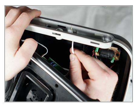
Guide the white button cables through the hole on the top of speaker case.
