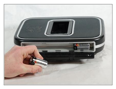
Once the door is open, use your hand to pull out the four batteries.
