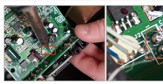
Desolder the two battery connections from the motherboard.
