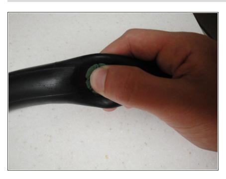
Apply pressure to the patch until the rubber cement is dry.
