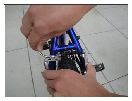
Squeeze the brake arms together and lift the brake cable from the caliper arms.
