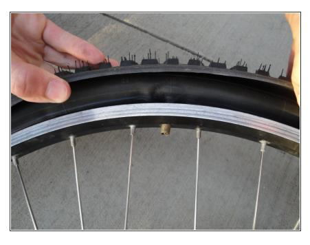
Remove the tube by pushing the valve through the hole in the rim and pulling out completely.
