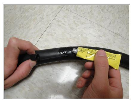
Apply rubber cement to an area around the hole that is bigger than the patch to ensure that the patch bonds completely.
