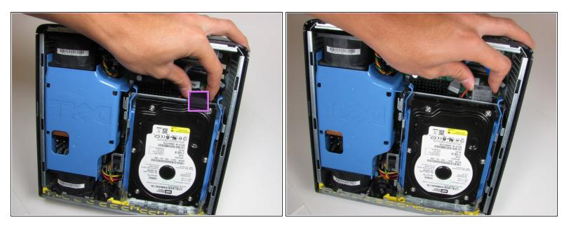
Unplug the power supply, distinguished by its red and yellow wires (yellow wire obscured from view).
