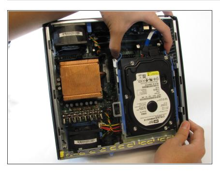
• Squeeze the release tabs on either side of the hard drive.
