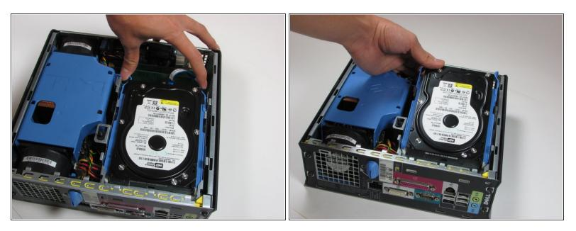
• Slide the Hard Drive out while squeezing the tabs.
