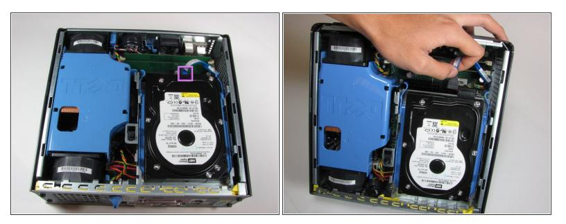
• Unplug the blue cable that connects the hard drive to the motherboard.
