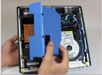
Remove the large blue cover from the computer, there are no screws or tabs keeping it in place.
