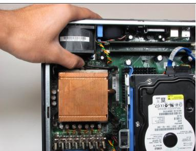
Press down on the release tab above the heat sink.
