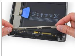
Slowly peel the upper component cable bracket up out of the iPad—leaving the tape pieces on the bracket to make it easier to reinstall.
