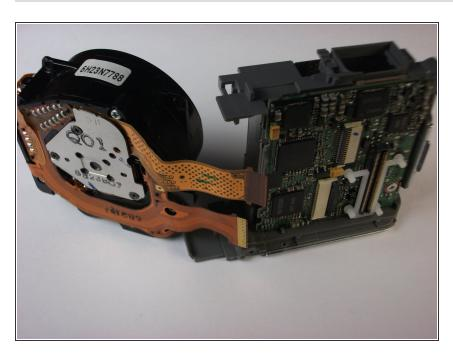
Remove the lens assembly as shown.
