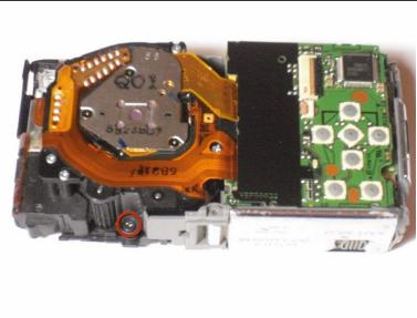
Remove the three black 5mm screws attached to the lens frame.
