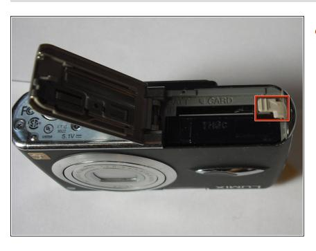
Open the battery latch, and slide the battery release lever to the right.
