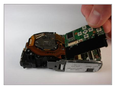
• Lift out the circuit board as shown.
