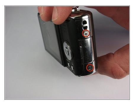
Remove the two 3.2 mm screws on the right side of the camera using a Phillips #00 screwdriver.
