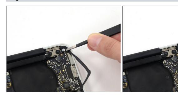
Remove the small rubber gasket from the corner of the upper case nearest the I/O board.
