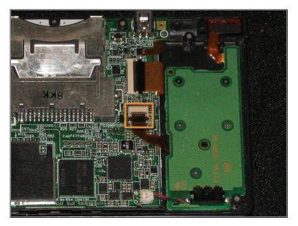
Flip up the black latch and disconnect the D-Pad/Power Button ribbon cable.
