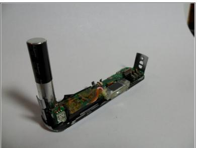
Replace the Flash Top Assembly with a new one.
