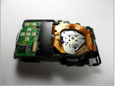
Carefully pry the Flash Top Assembly away from the top.
