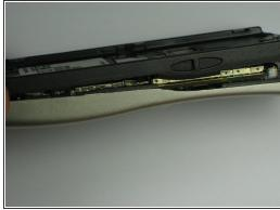
• Insert a plastic opening tool between the faceplate and the black backplate. Gently pry them apart, working from the lower end to the upper side of the phone.
