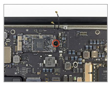
Remove the single 2.9 mm T5 Torx screw securing the AirPort/Bluetooth card to the logic board.
