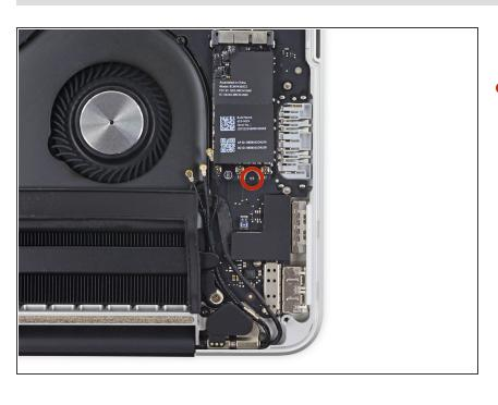
Remove the single 2.7 mm T5 Torx screw securing the AirPort board to the I/O board.
