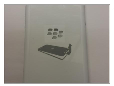
Remove the battery cover by grabbing the notch under the bottom speakers and lifting.
