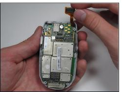
Separate the front ribbon cable from the board with a plastic opening tool.
