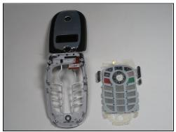
With the phone flipped open, peel the keypad back to remove it from the casing, starting from the bottom.
