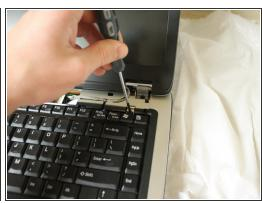
• Remove the two 3.67 mm screws from the top corners of the keyboard.
