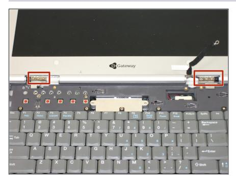
Using the Phillips #0 screwdriver, remove six screws that hold the LCD to the hinge.
