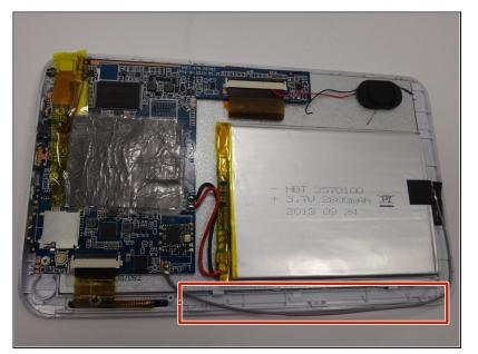
Locate the gray cord attached to the motherboard and the battery. This is the wifi antenna.
