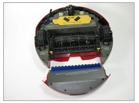
Slide out back bin by pressing the unmarked button on top of the Roomba.
