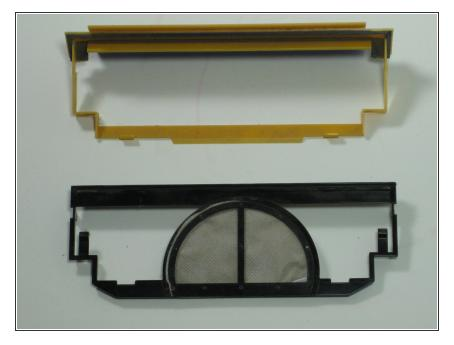
• Thoroughly clean or replace the air filter. This can be done with compressed air or by rinsing it with water.
