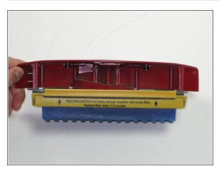
Reassemble the air filter assembly and slide the particle bin back into place
