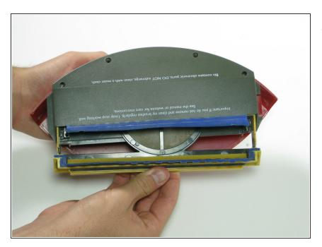
Slide out yellow bar on particle bin to access filter
