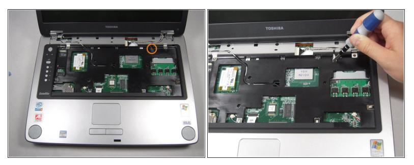
• Remove the 3.76mm screw from the ground wire.
