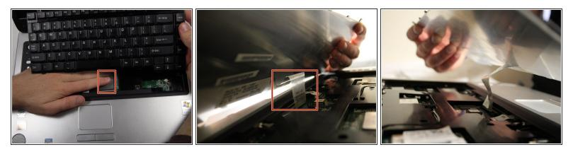
• Remove the cable connecting the keyboard with the motherboard.
