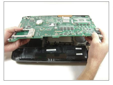
• Lift the motherboard's front edge up and then slide it forward.
