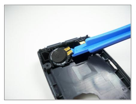
• Use a plastic opening tool to lift the speaker out of the back case.
