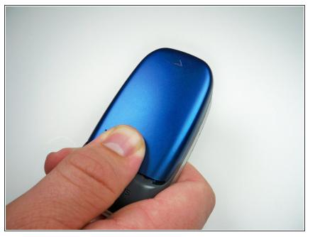
To remove the back cover, use your thumb to press down on the center of case and slide it off.
