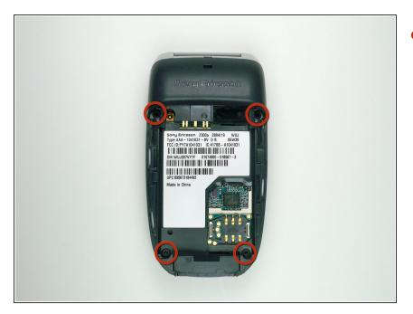
• To remove the back case first remove the four screws shown with a T5 Torx screwdriver
