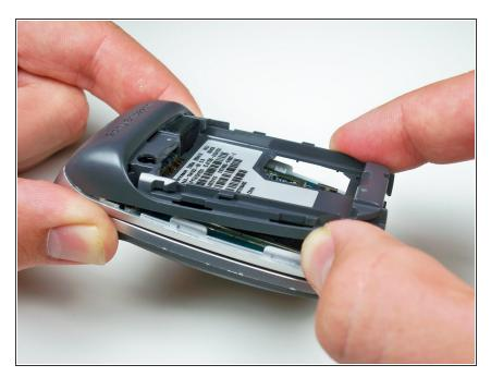
• Lift up towards the bottom and slide the case off.
