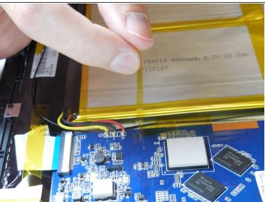
Remove the adhesive tape from the power connection cables.
