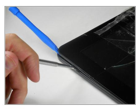
Wedge the plastic opening tool between the screen and the back panel to prevent re-engagement
