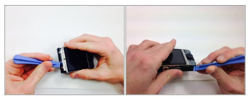
• Use a plastic opening tool to gently release the two indicated tabs.
