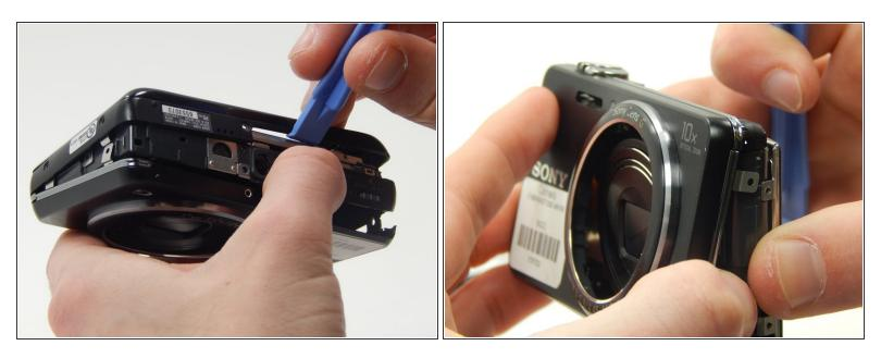
• Use the plastic opening tool to gently remove the front and back plates of the camera.
