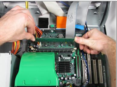
Push out on the cream colored tabs on each side of each RAM module until it pops up and out of its slot and remove the RAM.
