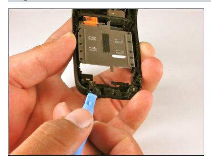
Use the plastic opening tool to pry out the microphone from the bottom of the compartment.
