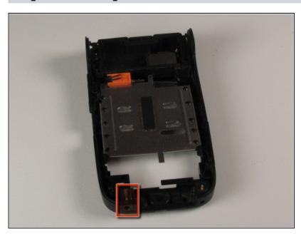
Locate the small speaker module on the back of the separated battery compartment in the lower left hand corner.
