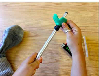
Spread a very thin layer of the melted glue on the basket end of the pole, then press on the new basket.
