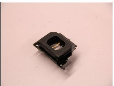
With the screws removed, the eyepiece can easily be pulled free.
