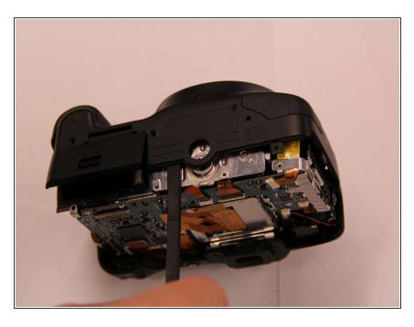
Using the spudger and plastic opening tool, pry the bottom of the front panel of the camera over the tripod mount.
