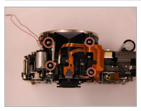
Remove the 4 screws holding the mirror box in place.
