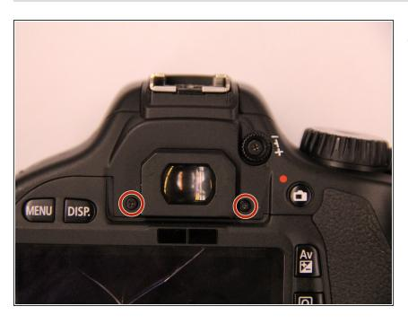
Remove the two screw beneath the eyepiece
