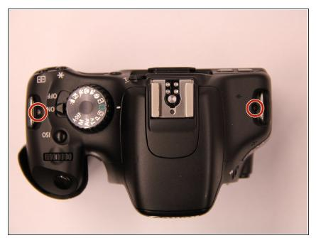
On the top cover, remove the two screws from under the metal tabs that are used to attach the camera straps.
