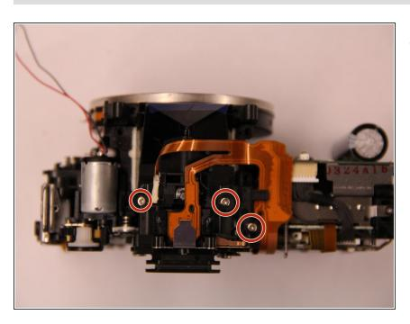
Remove 3 screws to disconnect the ribbon mount assembly
